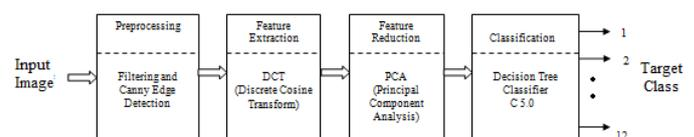
Fig.3. Block Diagram of the proposed vowel recognition system
