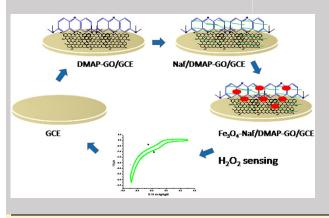
An unprecedented and highly selective non-enzymatic electrochemical sensor is developed on glassy carbon electrode with  $Fe_3O_4$  decorated Naf/DMAP linked graphene oxide ( $Fe_3O_4$ -Naf/DMAP-GO) nanohybrid film via electrostatic interaction of cationic organic compound with negatively charged oxygen containing groups (- $COO^-$  and -O) available on the edge of graphene oxide (GO).
