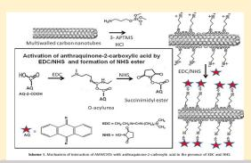
We have reported a simple, low cost and green preparation of nanowires of (anthraquinone-2-carboxylic acid/amino functionalized) multiwalled carbon nanotubes (HOOC-2-AQ/AMWCNTs) which has been further employed for the development of highly sensitive oxygen sensor. The prepared composite has been characterized by TEM and electrochemical studies.
