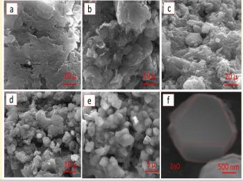
A novel approach was reported for the fabrication of polyaniline/ZnO-anchored bio-reduced graphene oxide nanocomposite *via in-situ* chemical polymerization of aniline doped with bio-reduced GO and ZnO through  $\pi$ -  $\pi$  interaction and electrostatic interaction.
