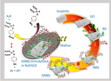
The synthesis of AuNPs/neutral red-biofunctionalized graphene is reported and demonstrated as efficient platform for sensitive detection of hazardous organophosphate pesticide 'Methyl Parathion' via reduction of -NO<sub>2</sub> group.
