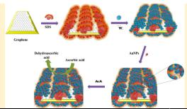
A rapid and sensitive tailor-made electrode based on the gold nanoparticles (AuNP's) modulated hydrophilic sodium dodecylsulphate (SDS) wrapped graphene (G)-Tolonium chloride (TC) (GSTG) nanocomposite was designed step-by-step in an easy and green way for the detection of ascorbic acid (AcA).
