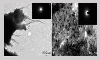
A multi-walled carbon nanotube composite electrode incorporating Polyaniline (PANI) and Polyacrylic acid (PAA) is presented by diffusing aniline and PAA into Nafion-MWCNTs membranes supported upon a platinum macro disc electrode. Nafion is found to be an ideal medium for dispersion of MWCNTs and for the formation of a homogeneous composite. The composite has been characterized utilizing SEM, TEM, FT-IR and electrochemical techniques.
