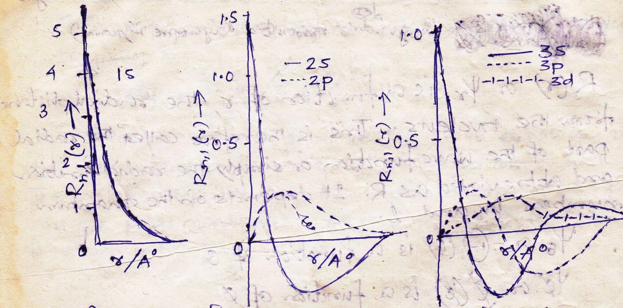
\* Variation of the R function with  $r$  for various hydrogen orbitals
